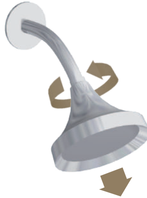
Fig. 1 Unscrew shower head from pipe fixture.
