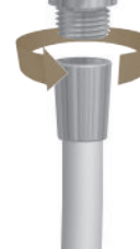
Fig. 2 Screw the shower hose onto the bottom of the Elixator
