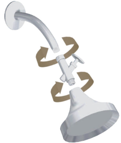
Fig. 2 Screw the Elixator onto the pipe fixture. Screw the shower head onto the bottom of the Elixator
